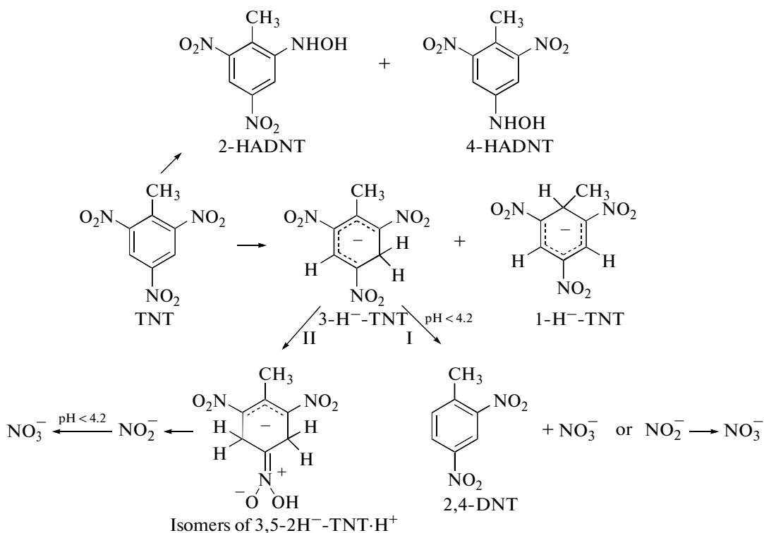
**Fig. 3.** Proposed pathways of TNT transformation by *G. candidum* AN-Z4. Roman numerals designate two possible variants of the xenobiotic degradation.
